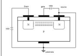
In fig. both V<sub>GS</sub> & V<sub>DS</sub> have been set at positive with respect to the source. The positive potential at the gate will attract the electrons from the P substrate & accumulate in the region near to the surface of  $SiO_2$  layer. The  $SiO_2$  layer & its insulating qualities will prevent the negative carriers (i.e. electrons) from being absorbed at the gate.
